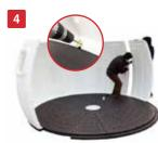
Connect all the lower wall panels. Fasten the lower panels to the floor panel with screws.
